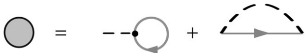
FIGURE 3 | Feynman diagrams for the Hartree–Fock self-energy. The dashed line represents the bare Coulomb interaction, and the arrow a one-body Green's function. The arrow closed as a circle is the density Eq. (3) (the diagonal of the Green's function Eq. (8)). The first contribution is the Hartree potential, and the second contribution is the exchange self-energy.
