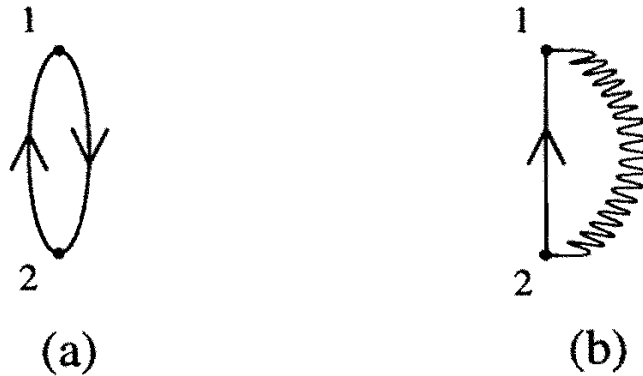
Fig. 12. (a) Diagrammatic representation of the Random-Phase approximation (RPA) for the polarisation function P , and (b) of the dynamically-screened exchange, or GW , approximation for the self-energy operator. The directed solid line from j to i stands for the single-particle Green function G(i, j) and the wavy line for W (whence the “ GW ” approximation). If the solid line is taken to represent G_0 , the single-particle Green function pertaining to some “non-interacting” Hamiltonian, then diagram (a) represents the exact density-density correlation function \chi_0 of the corresponding “non-interacting” system. In the main text, by \chi_0 we denote the density-density response function pertaining to the “non-interacting” Kohn-Sham Hamiltonian.
