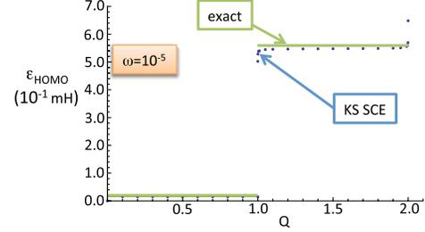
FIG. 4 (color online). Self-consistent results for the spin-restricted KS HOMO eigenvalue as a function of the particle number  $Q$  for a three-dimensional electronic system in the external harmonic potential,  $v_{\text{ext}}(\mathbf{r}) = (1/2)\omega^2 r^2$ , with  $\omega = 10^{-5}$ . The KS SCE results are compared with the exact chemical potential  $E_{N+1} - E_N$  [60,61].
