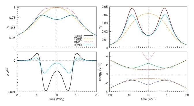
FIG. 4. (Color online) Time dependence of the one-matrix for the linear-time potential,  $\tau = 2$ , U = 4. Shown are  $\gamma_1$  (top left),  $\gamma_2$  (top right),  $A - A^{(0)}$  (bottom left), and adiabatic energies (bottom right). Energies are the same as in Fig. 2 with the addition of HF eigenvalues (dashed lines).
