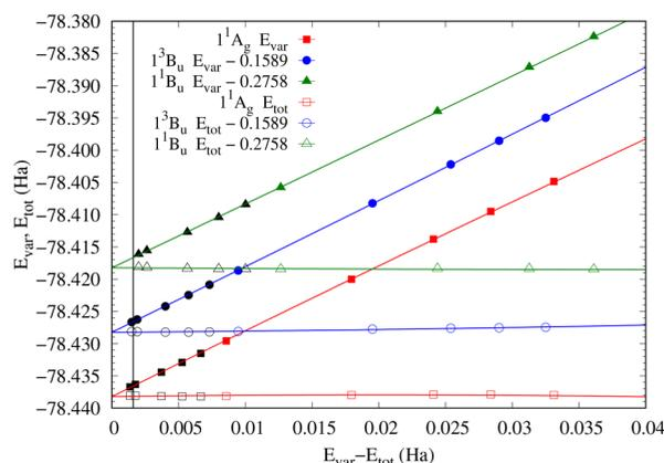
**Figure 2.** Fit of variational and total energies of ethylene using all data points. The black line is placed at 1.6 mHa. States are separated from one another by 0.01 Ha for clarity. The tightest SHCI calculation used  $\epsilon_V = 7 \cdot 10^{-6}$  Ha. The extrapolated energies obtained using all data points are compared to those obtained by omitting the black points in **Table 3**.
