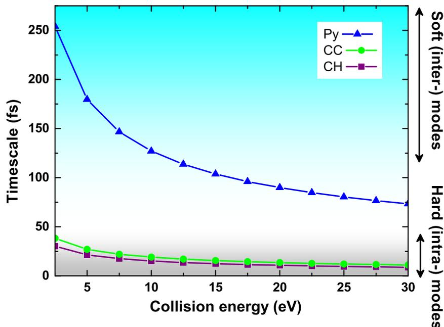
**Figure 4.35:** Timescales, as a function of center of mass collision energy, for argon to travel across some typical distances: a carbon-carbon bond (green), a carbon-hydrogen bond (purple) or the largest axis of the pyrene molecule (blue).
