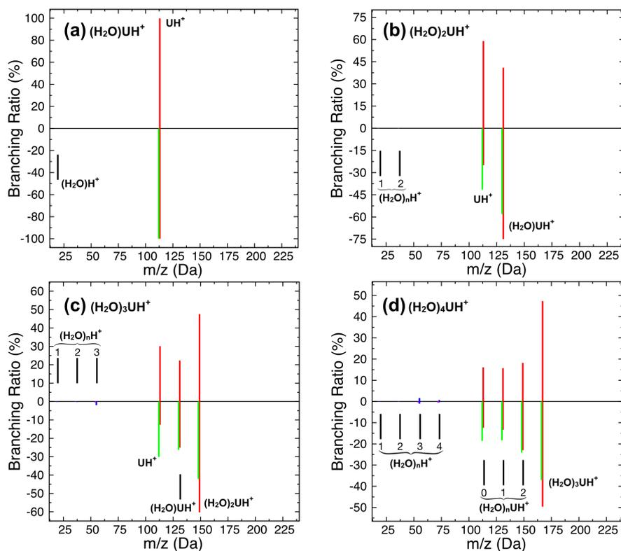
**Figure 4.20:** Simulated mass spectra (positive area) of the charged fragments after 15 ps simulation time (fragments  $(\text{H}_2\text{O})_n\text{H}^+$  in red and  $(\text{H}_2\text{O})_n\text{UH}^+$  in blue for argon;  $(\text{H}_2\text{O})_n\text{H}^+$  in pink and  $(\text{H}_2\text{O})_n\text{UH}^+$  in green for neon) from isomers (a) 1a, (b) 2b, (c) 3b, (d) 4b. The counterparts in experiment are plotted (negative area).
