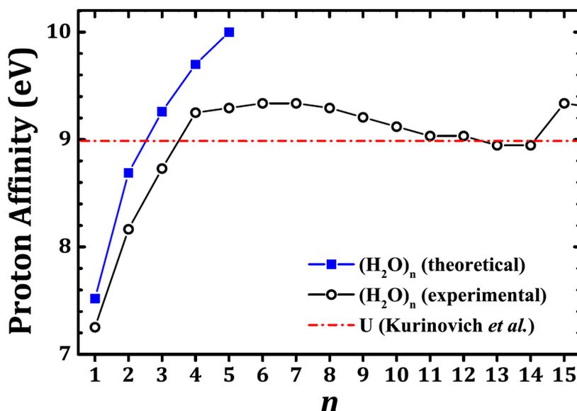
**Figure 3.16:** The proton affinities of water clusters as a function of the number of water molecules  $n$ , which are taken from the work of Magnera (black circles) [411] and from the work of Cheng (blue squares).[412] The value of the proton affinity of uracil (red dotted dashed line) is also plotted.[410]
