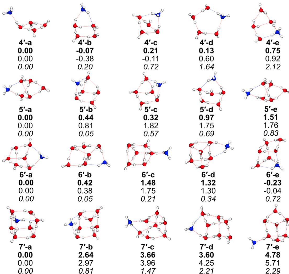
**Figure 3.10:** The first five low-energy isomers of cluster  $(\text{H}_2\text{O})_{4-7}\text{NH}_3$  and the associated relative energies (in  $\text{kcal}\cdot\text{mol}^{-1}$ ) at MP2/Def2TZVP level with (bold) and without ZPVE correction and SCC-DFTB level (italic).
