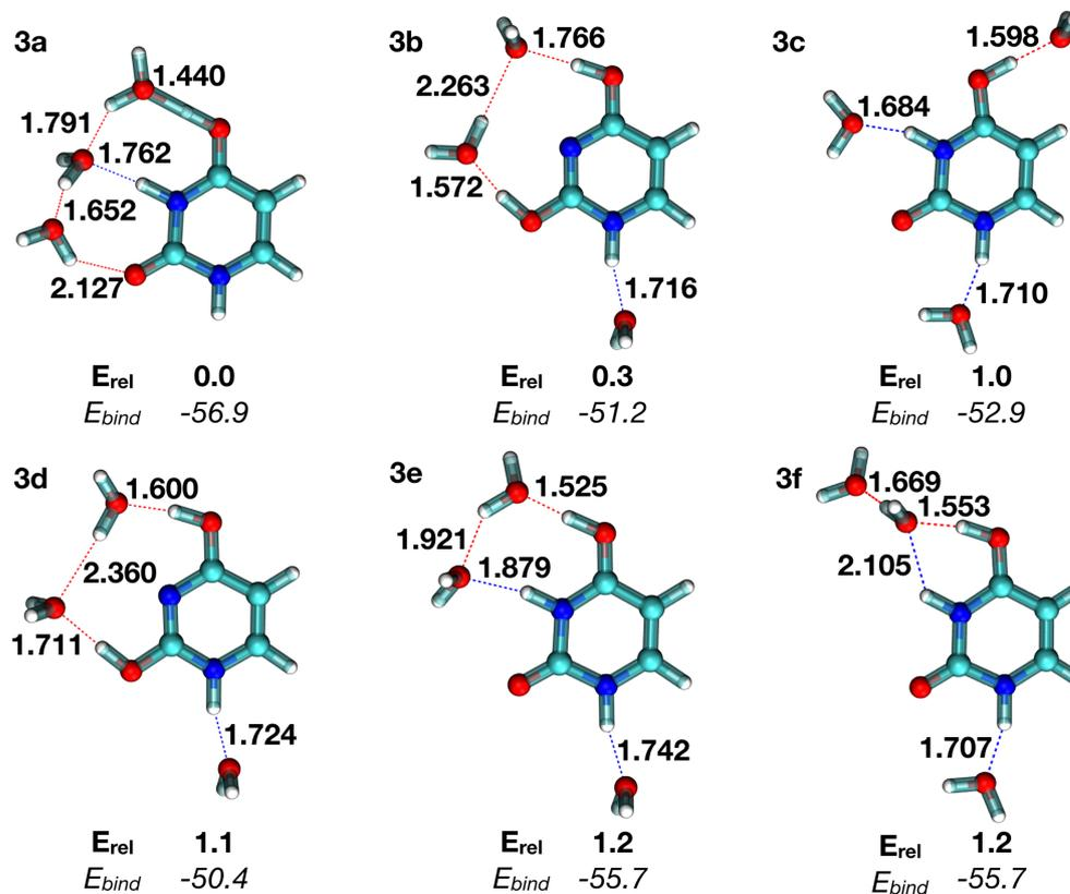
**Figure 3.20:**  $(\text{H}_2\text{O})_3\text{UH}^+$  lowest-energy structures obtained at the MP2/Def2TZVP level of theory. Relative ( $E_{rel}$ ) and binding energies ( $E_{bind}$ ) are given in kcal.mol<sup>-1</sup>. Important hydrogen-bond distances are indicated in bold and are given in Å.
