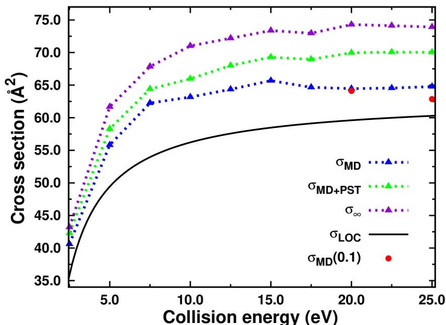
**Figure 4.29:** Dissociation cross sections of  $\text{Py}_2^+$  after collision with argon as a function of center of mass collision energy for the short (MD), experimental (MD+PST) and infinite timescales. Cross sections resulting from the LOC model are also plotted.  $\sigma_{\text{MD}}(0.1)$  denotes the dissociation cross section for short (MD) timescale with a time step of 0.1 fs.
