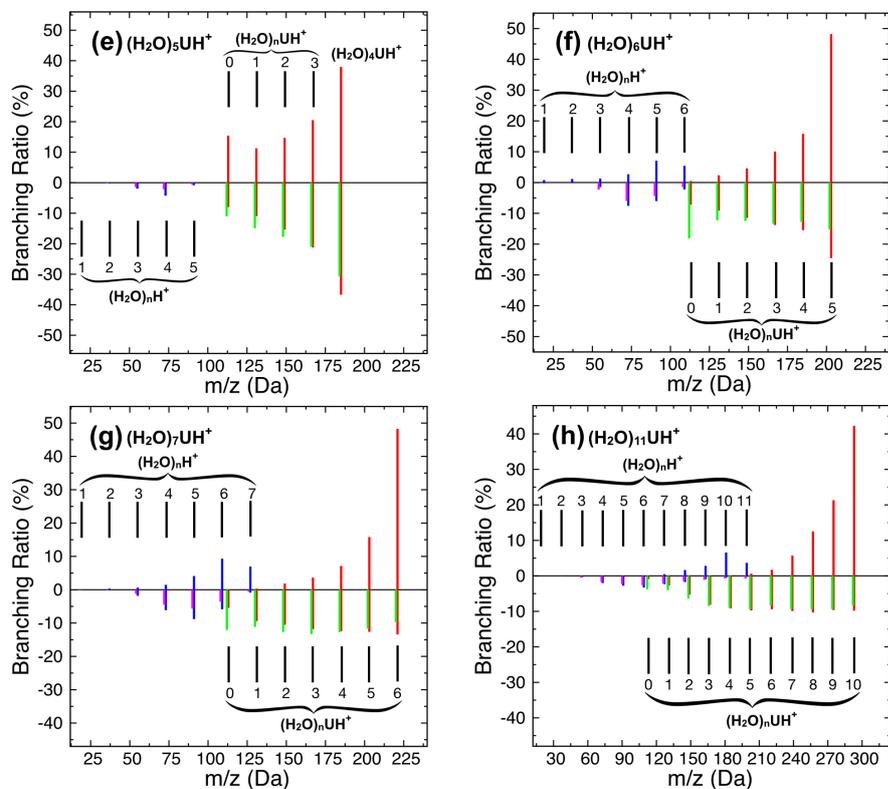
**Figure 4.21:** Simulated mass spectra (positive area) of the charged fragments after 15 ps simulation time (fragments  $(\text{H}_2\text{O})_n\text{H}^+$  in red and  $(\text{H}_2\text{O})_n\text{UH}^+$  in blue) from isomers (e) 5d, (f) 6f, (g) 7d, and (h) 11d. The counterparts in experiment are plotted (negative area).
