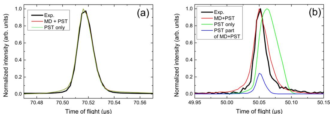
**Figure 4.24:** Normalized time of flight mass spectra of the parent pyrene dimer cation (a), and the pyrene fragment  $Py^+$  (b) resulting from the collision of  $Py_2^+$  with argon at a center of mass collision energy of 17.5 eV. The black line is for the experimental result whereas red and green curves are the MD+PST and PST model results. The blue curve is the PST subcontribution of the MD+PST model.
