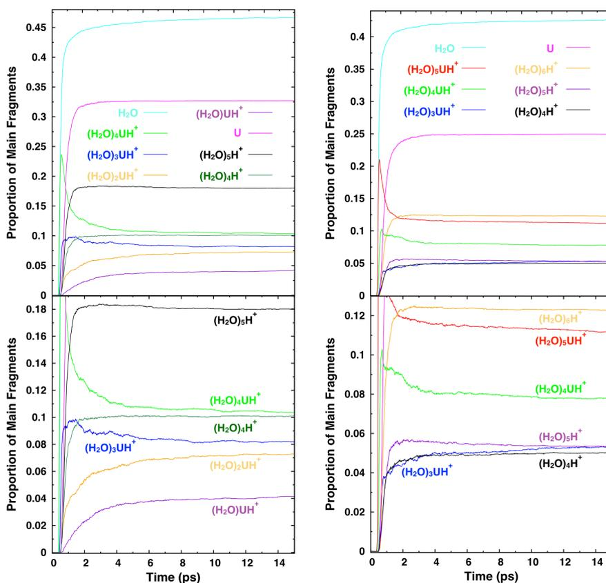
**Figure 4.8:** Time-dependent proportions of the main fragments obtained from the dissociation of the lowest-energy isomers of  $(\text{H}_2\text{O})_5\text{UH}^+$  (left) and  $(\text{H}_2\text{O})_6\text{UH}^+$  (right). Bottom panels correspond to a zoom over the lower proportions.
