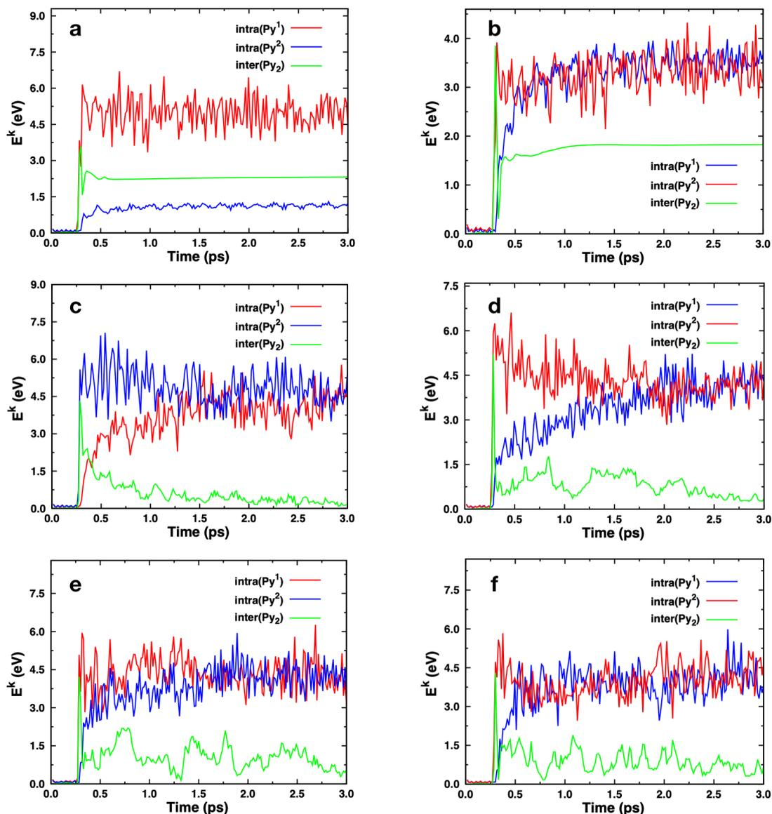
**Figure 4.37:** Instantaneous kinetic energies as a function of time for intra and intermolecular modes of the pyrene dimer at a collision energy of 22.5 eV. Impact parameters  $b$  are (a) 2, (b) 3, (c) 0, (d) 2.5, (e) 2, and (f) 2 Å. In cases (a) and (b), dissociation takes place whereas in the other cases the dimer remains undissociated at the end of the MD simulation.
