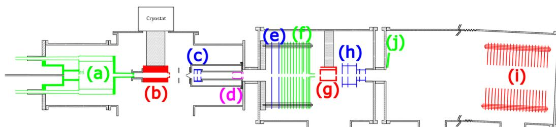
**Figure 4.1:** Schematic view of the experimental setup. (a) Cluster gas aggregation source. (b) Thermalization chamber. (c) First Wiley–McLaren acceleration stage. (d) Massfilter. (e) Energy focusing. (f) Deceleration. (g) Collision cell. (h) Second Wiley–McLaren acceleration stage. (i) Reflectron. (j) Micro-channel plate detector.
