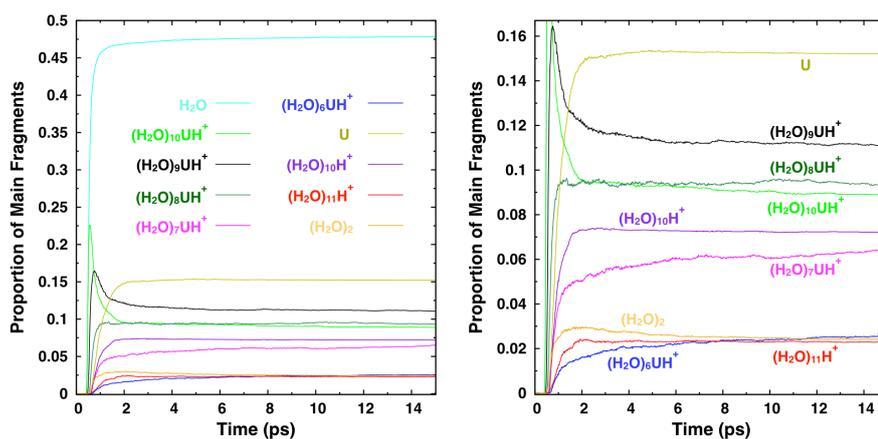
**Figure 4.9:** Time-dependent proportions of the main fragments obtained from the dissociation of the lowest-energy isomer of  $(\text{H}_2\text{O})_{11}\text{UH}^+$ . Right panel corresponds to a zoom over the lower proportions.
