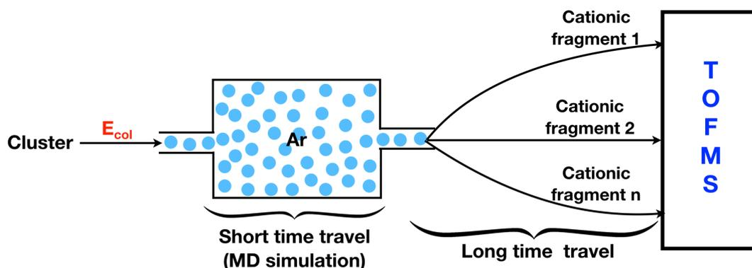
Figure 4.2: Schematic of the simplified experimental setup.
