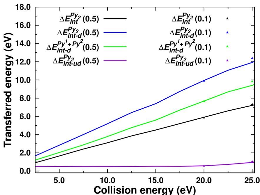
**Figure 4.30:** At the end of the MD collision simulations with a time step of 0.1 and 0.5 fs, the total transferred energy  $\Delta E_{int}^{Py_2}$  to the rovibrational modes or restricted to the sole dissociated ( $\Delta E_{int-d}^{Py_2}$ ) or undissociated ( $\Delta E_{int-ud}^{Py_2}$ ) pyrene dimers as a function of collision energy. The transferred energy to the monomers rovibrational modes for the dissociated dimers  $\Delta E_{int-d}^{Py_1+Py_2}$  is also plotted.
