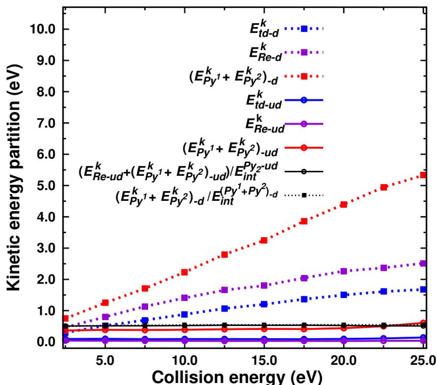
**Figure 4.34:** Kinetic energy partition for dissociated (-d) and undissociated (-ud) trajectories at the end of the MD simulation as a function of collision energy.
