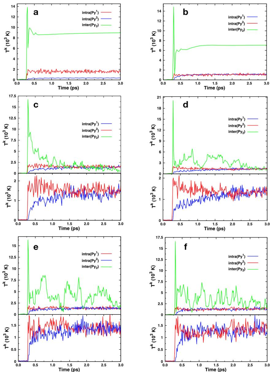
**Figure 4.36:** Instantaneous kinetic temperatures as a function of time for intra and intermolecular modes of the pyrene dimer at a collision energy of 22.5 eV. Impact parameters  $b$  are (a) 2, (b) 3, (c) 0, (d) 2.5, (e) 2, and (f) 2 Å. In cases (a) and (b) dissociation takes place whereas in the other cases the dimer remains undissociated at the end of the MD simulation. In (c) to (f) the lower panel is a vertical zoom of the corresponding intramolecular parts in upper panel.
