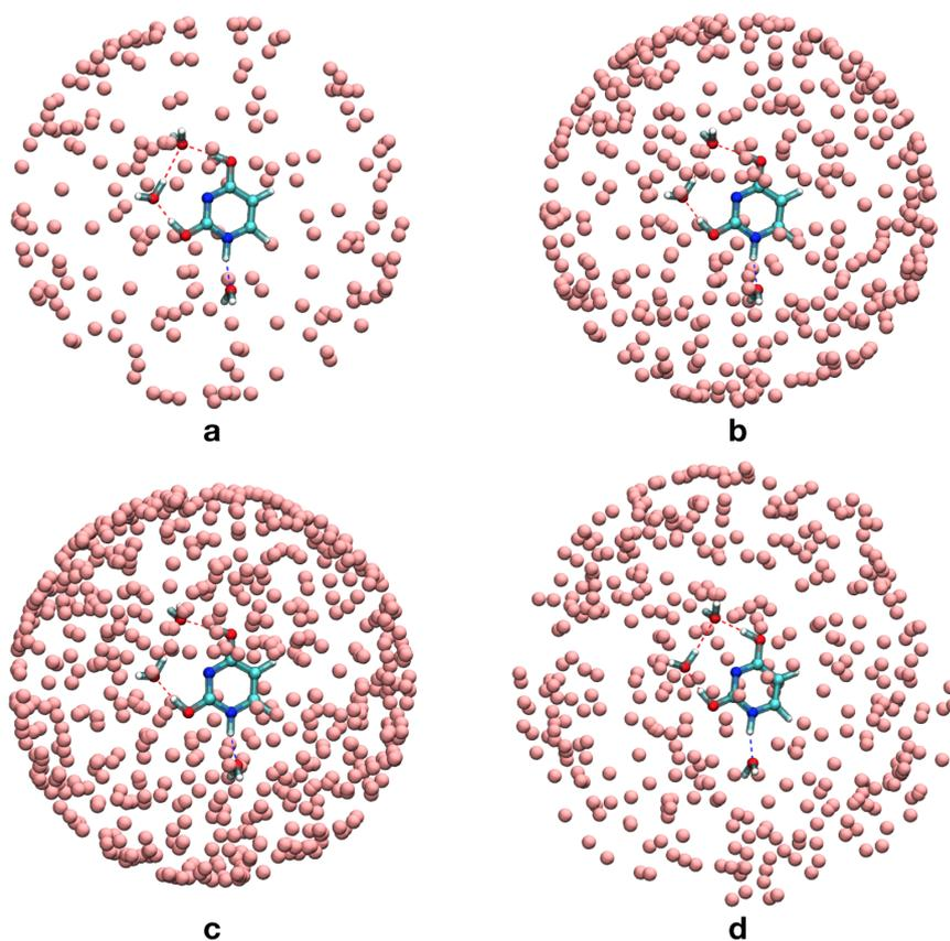
**Figure 4.4:** Schematic representation of random argon orientations for the collision with the second lowest-energy isomer of cluster  $(\text{H}_2\text{O})_3\text{UH}^+$ . 200 (a), 400 (b) and 600 (c) random argon orientations are generated with impact parameter being 0. 200 orientations are generated with impact parameter being 0 and 6 (d), respectively.
