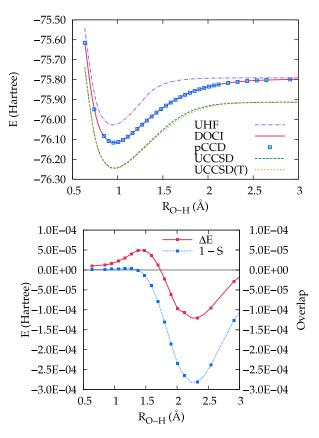
FIG. 5. Symmetric double dissociation of H<sub>2</sub>O. Top panel: Dissociation energies from DOCI and pCCD, as well as from UHF and CCSD and CCSD(T) based thereon. Bottom panel: Errors in the energy ( $\Delta E$ , defined in Eq. (27) and measured on the left axis) and in the overlap (1-*S*, measured on the right axis with *S* defined in Eq. (28)).
