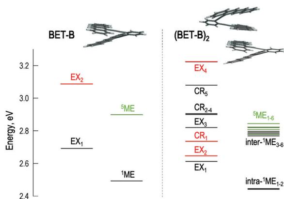
Fig. 12 Energy levels of BET-B (left) and (BET-B)<sub>2</sub> (right) computed at the RAS-SF/cc-pVDZ level. Energies were corrected by means of excited state decomposition analysis.<sup>80</sup> Dark, bright and quintet states marked in black, red and green, respectively. EX: excitonic state; CR: charge resonance; ME: multiexcitonic state.
