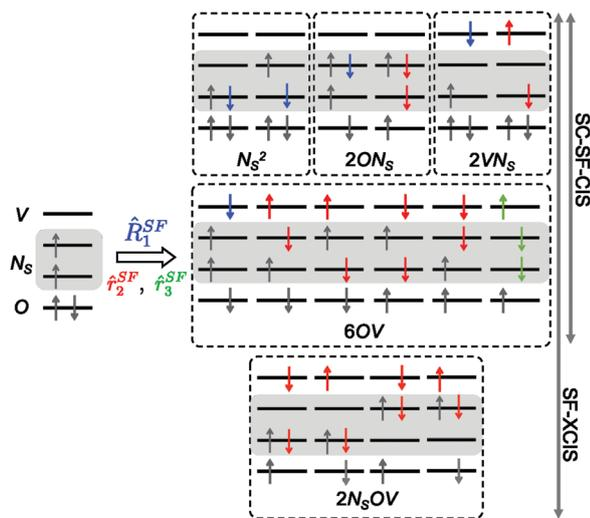
**Fig. 11** Electronic configurations generated in the SC-SF-CIS and SF-XCIS methods through the full spin-flip single excitation operator (blue), a subset of the two- (red) and three-electron (green) spin-flip excitations with one spin-flip excitation applied to a high-spin triplet.  $N_s$ ,  $O$ , and  $V$ : singly occupied (highlighted in grey), doubly occupied and fully virtual orbitals at the reference state. The dimension of each type of configuration subspace is indicated at the bottom.
