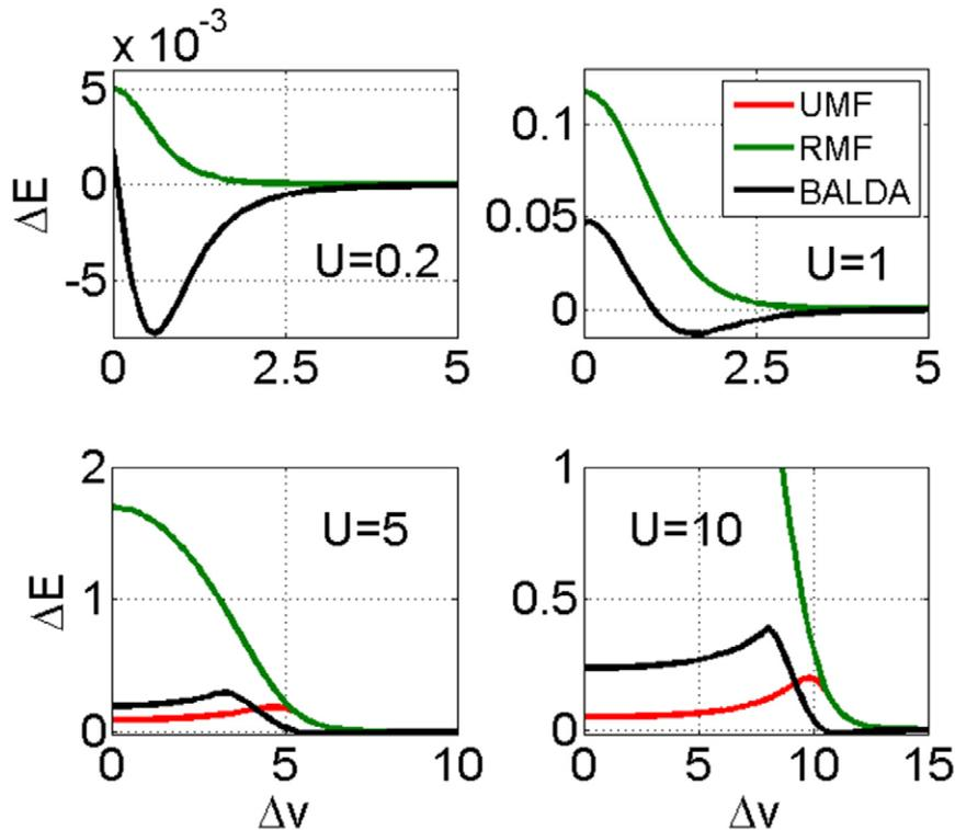
**Figure 27.** Plots of the RMF, UMF, and BALDA  $\Delta E = E^{\text{approx}} - E^{\text{exact}}$  as a function of  $\Delta v$  for  $U = 0.2, 1, 5,$  and  $10$ . For small  $U$  the RMF and UMF results are indistinguishable. Here  $2t = 1$ .
