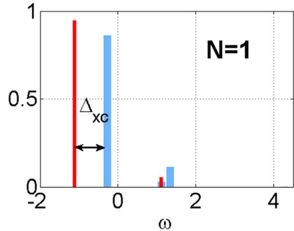
**Figure 17.** Spin- $\downarrow$  resolved spectral function for  $N = 1$  and  $U = 1$ ,  $\Delta v = 2$ , ( $2t = 1$ ). Here  $I = 1.12$ ,  $A = 0.27$ , and  $\epsilon^{\text{LUMO}} = \epsilon^{\text{HOMO}} = -1.12$ .
