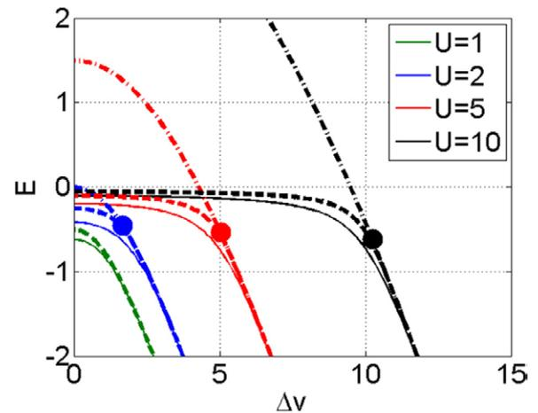
**Figure 25.** Ground-state energy of the unrestricted Hartree–Fock (thick dashed line), restricted Hartree–Fock (dot dashed line), and exact ground-state (thin solid line) of the Hubbard dimer as a function of  $\Delta v$  for several values of  $U$  and  $2t = 1$ . The dot shows the Coulson–Fischer point at which the symmetry breaks spontaneously. For smaller  $\Delta v$  the UHF energy is below RHF while for larger  $\Delta v$  they are the same.
