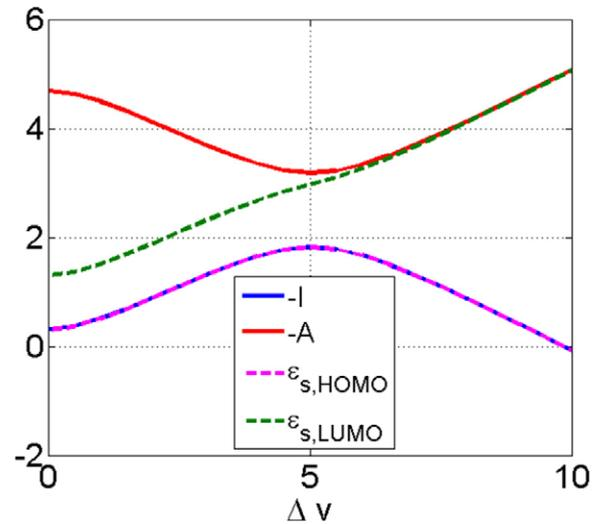
Figure 12. Plot of  $-A$ ,  $-I$ ,  $\epsilon^{\text{HOMO}}$ , and  $\epsilon^{\text{LUMO}}$  as a function of  $\Delta v$  with  $U = 5$  and  $2t = 1$ .
