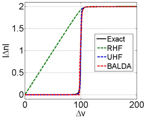
**Figure 32.** Plots of  $\Delta n$  in HF and BALDA as a function of  $\Delta v$  for  $U = 100$  ( $2t = 1$ ). The crossover from the charge-transfer to the Mott–Hubbard regime happens at about  $U \approx \Delta v$ .
