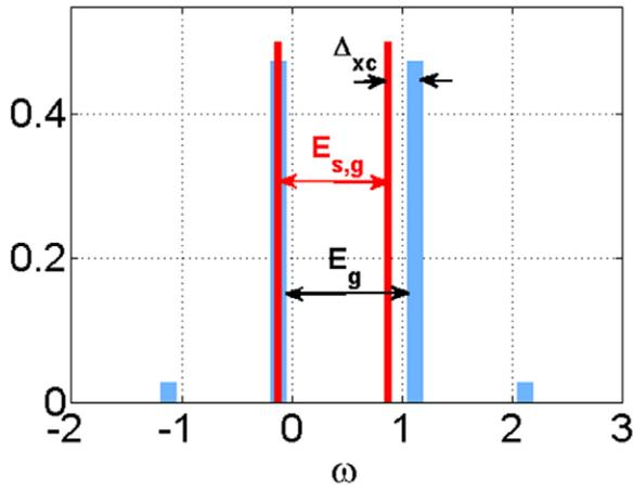
**Figure 13.** Spectral function of symmetric dimer for  $U = 1$ ,  $\Delta v = 0$ , and  $2t = 1$ . The physical MB peaks are plotted in blue, the KS in red. Here  $I = 0.1$ ,  $A = -1.1$ , and  $\epsilon^{\text{LUMO}} = 0.9$ , corresponding to  $\Delta v = 0$  in figure 11.
