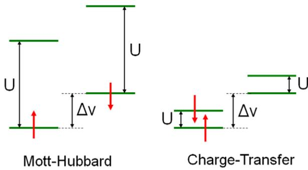
**Figure 1.** Many-body view of two distinct regimes of the asymmetric Hubbard dimer. On the left, the charging energy is much greater than the difference in on-site potentials. On the right, the situation is reversed.
