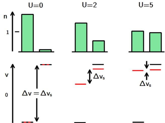
**Figure 2.** DFT view: occupations  $n$  and potentials  $v$  of an asymmetric half-filled Hubbard dimer as a function of  $U$ . The on-site potential difference  $\Delta v$  is shown in black and the KS on-site potential difference  $\Delta v_s$  is in red. The second and third panels correspond to the situations of figure 1.
